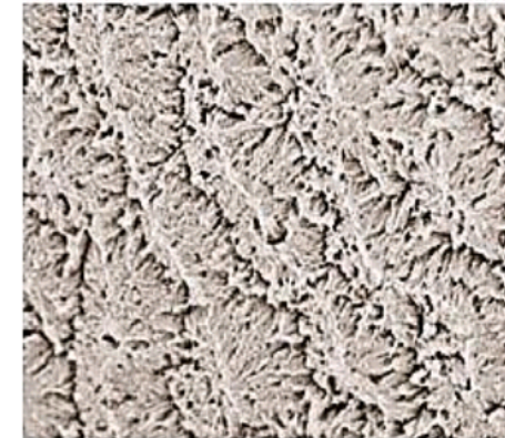
Enamel after 37 % phosphoric acid etching
